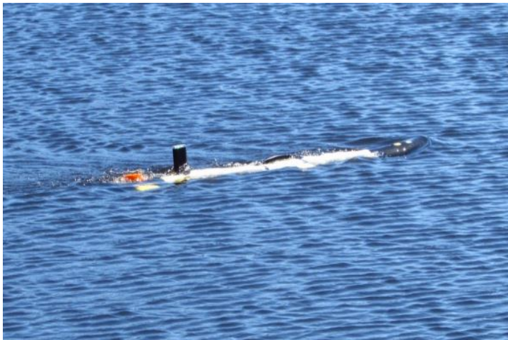
Figure 2 An Iver2-580 with Klein UUV3500 side scan sonar, underway during testing
