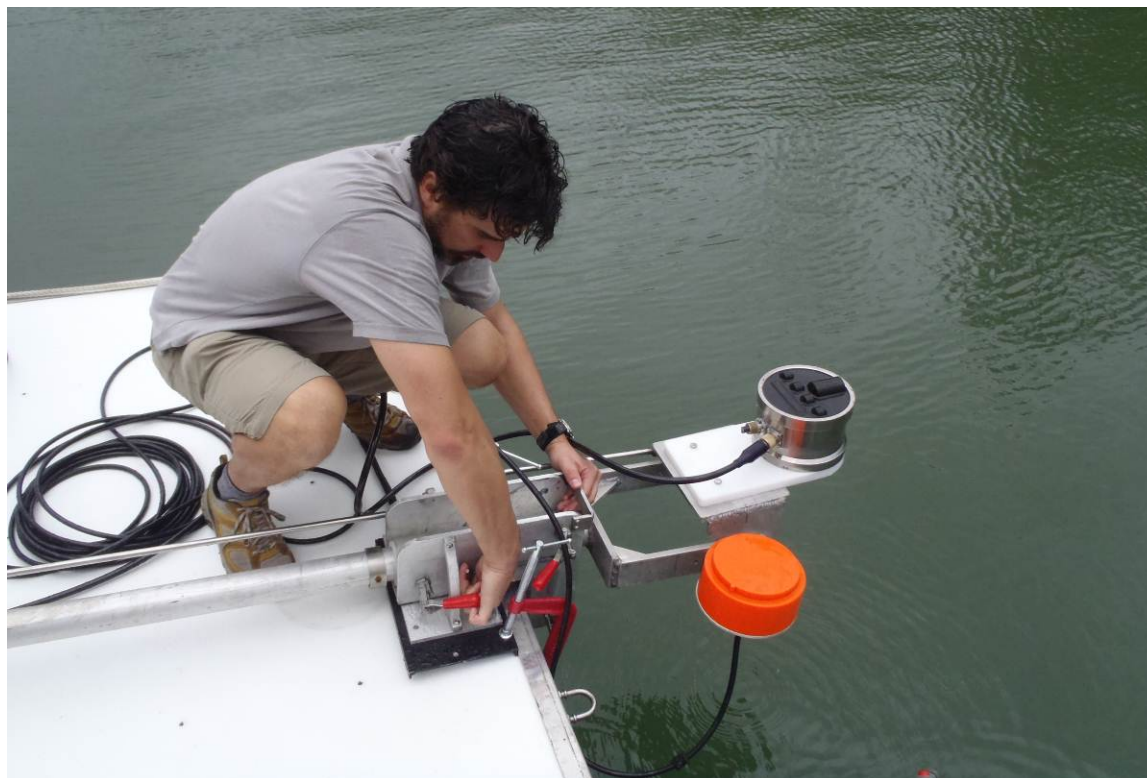
Chris Taylor (NOAA NCCOS Beaufort, NC) prepares a flexible overboard mount for deploying the Mesotech M3 multibeam sonar and Simrad EK60 splitbeam transducer.
